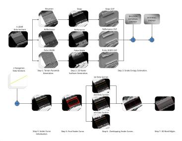
Fig. 1. Road edge extraction algorithm components [6].
