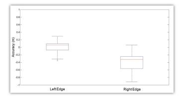
Fig. 12. Box plot for the accuracy values of the automatically extracted left and right edges in the second  $105 \mathrm{m}$  road section.
