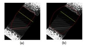
Fig. 4. Final position of the snake curve is represented in red over the slope raster surface with (a)  $\kappa_1=1$  and (b)  $\kappa_1=4$  parameter in 10 m national primary road section, while the navigation points are represented in yellow.
