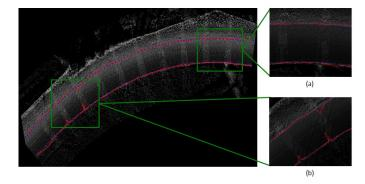
Fig. 10. The automatically extracted 3D edges are represented in red and the manually digitised 3D edges are represented in blue in the third 90m road section. The inset pictures (a) and (b) of left and right edges show some of the points in detail.
