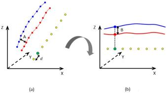
Fig. 6. Road edge validation approach: (a) Original and (b) rotated positions of extracted and reference road edges, where red represents the extracted road edges, blue represents the reference road edges, yellow represents the navigation points and green represents the navigation point selected in each iteration.
