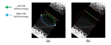
Fig. 5. (a) Initial and (b) final position of the snake curve is represented in red over the slope raster surface with  $\kappa_1^{left}=1$  and  $\kappa_1^{right}=4$  in a 10m national primary road section, navigation points are represented in yellow while end points of major axis of the initial snake curve are represented as white dots.
