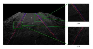
Fig. 8. The automatically extracted 3D edges are represented in red and the manually digitised 3D edges are represented in blue in the first 50m road section. The inset pictures of (a) left and (b) right edges show some of the points in detail.
