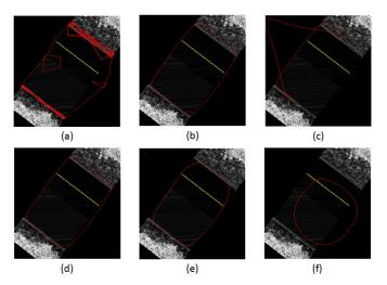
Fig. 2. Final position of the snake curve is represented in red over the slope raster surface in the (a) first, (b) second, (c) third, (d) fourth, (e) fifth, (f) sixth and (g) seventh test case of internal energy analysis, while the navigation points are represented in yellow.
