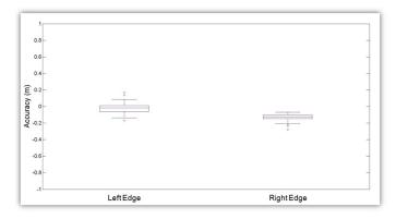
Fig. 11. Box plot for the accuracy values of the automatically extracted left and right edges in the first 50m road section.
