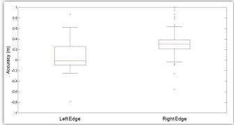
Fig. 13. Box plot for the accuracy values of the automatically extracted left and right edges in the third 90m road section.
