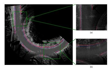
Fig. 9. The automatically extracted 3D edges are represented in red and the manually digitised 3D edges are represented in blue in the second 105m road section. The inset pictures (a) and (b) of left and right edges show some of the points in detail.
