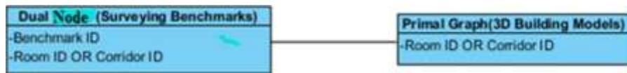
Fig. 5 Connection between surveying benchmarks and 3D building model based on their IDs
