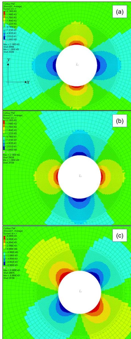
Fig. 2: Contour plot of stresses for an infinite composite plate containing a circular hole of radius 10mm under bi-axial loading (Val-A), i.e.  $N_x=N_y=280\text{N/mm}$ ; (a) Normal stress in x-direction, (b) Normal stress in y-direction and (c) Shear stress in xy plane
