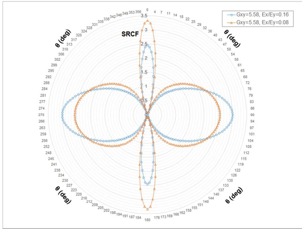
Fig. 7: Distribution of the SRCF around the edge of the hole for uni-axial loading for  $G_{xy}=5.58\text{GPa}$  for stacking sequences of  $(90)_{13}/0_s$  and  $(90)_{28}$  associated to  $E_x/E_y$  of 0.16 and 0.08, respectively. The load is applied at  $0^\circ$  direction
