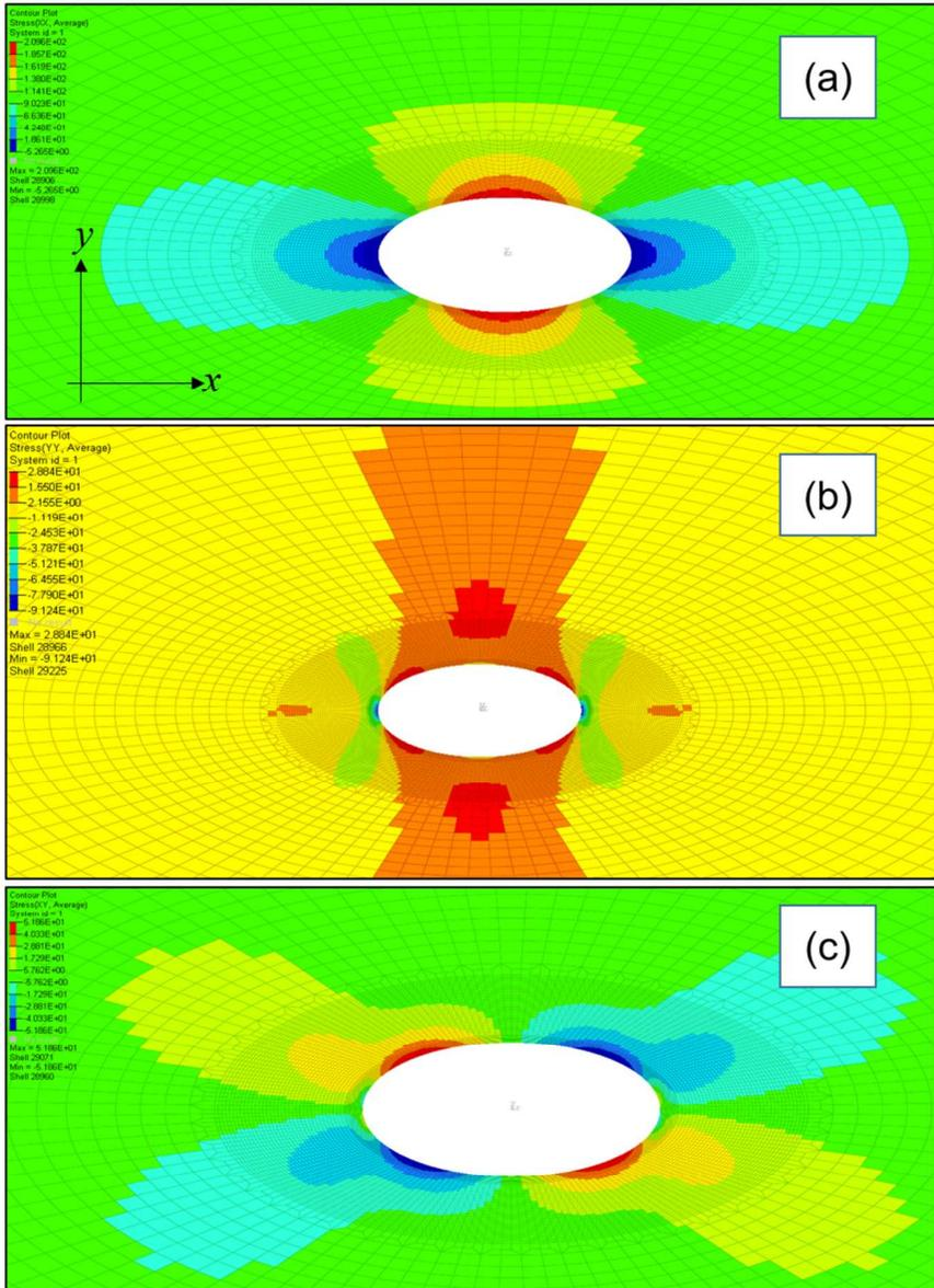
Fig. 3: Contour plot of stresses for an infinite composite plate containing an elliptical hole of radius 10mm under uni-axial loading (Val-B), i.e.  $N_x=280N/mm$ ; (a) Normal stress in x-direction, (b) Normal stress in y-direction and (c) Shear stress in xy plane
