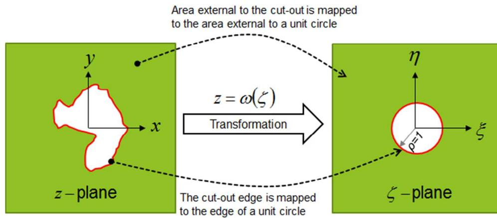
22 Fig. A1: Illustration of mapping a hole having an irregular shape in an infinite plate onto a unit circle using
