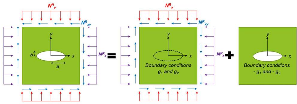
Fig. A2: Use of principle of superposition for calculation of stress functions
