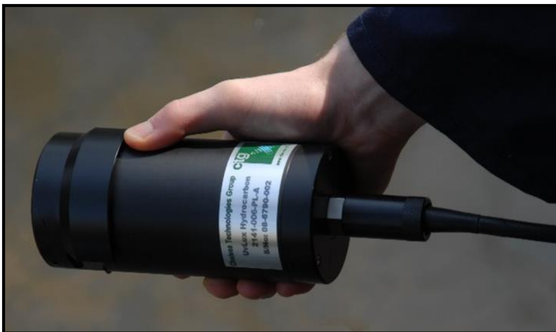
Figure 5.1: Image of the UviLux sensor (Chelsea Technologies Group Ltd., UK), complete with light cowl. Used with permission of the creator, Chelsea Technologies Group Ltd.
