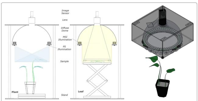
Fig. 2 Scanning set-up. Side-view diagram of apparatus set-up for canopy and PS imaging (left) and detached leaf assay with MSI (centre) showing the major system components with three-dimensional view (right)
