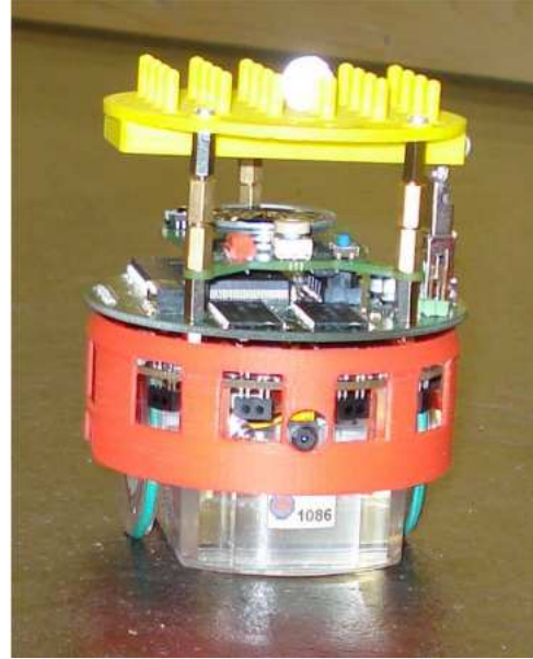
Figure 22. An e-puck with Linux board fitted in between the e-puck motherboard (lower) and the e-puck speaker board(upper). Note both the red skirt, and the yellow hat that provides a matrix of pins for the reflective spheres which allow the tracking system to identify and track each robot.
