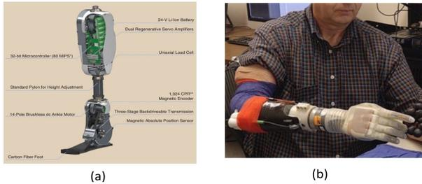
Fig. 6: Prototypes of the prostheses (a) A powered prosthesis with a hybrid controlled piecewise-passive impedance-based designed to provide level walking functionality for amputees [48], (b) The University of Utahs neuroprosthetic prosthetic arm which allows amputees to regain the sense of pressure, vibration, temperature, pain, and movements by creating a connection between their brain and a computer [49].
