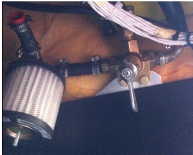
Figure 4.2: Part of the modified suction system located in the right-hand leg room of the cockpit (photograph taken by the Author)
