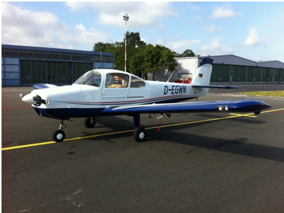
Figure 7.2: Fuji FA 200 – 160, single-engine, low-wing aeroplane with a conventional tail and fixed landing gear. Note: that this aircraft was instrumented for experimental spin tests. It is owned by TFF GmbH.
