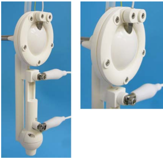
Figure 3. Bio-actuator 3D printed working prototype.
