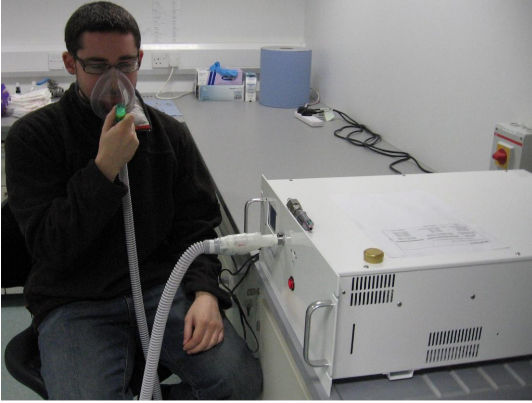
Figure 2.1. Breath ammonia measurement using photoacoustic spectroscopy. The typical procedure for volunteer breath collection using the Nephrolux TM .
