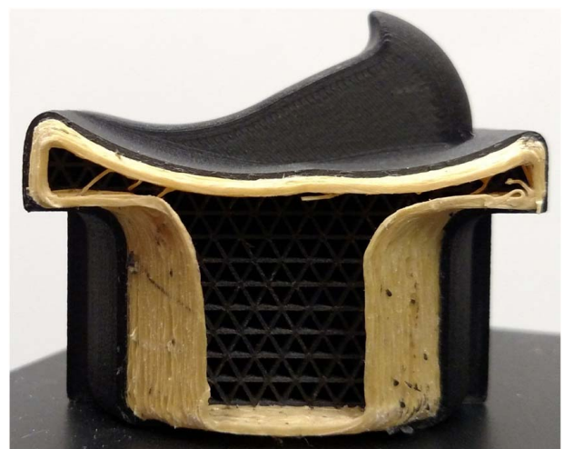
Fig. 10 Side view of a 3D print where the outer nylon/carbon fiber layer has been removed to expose the Kevlar layer underneath
