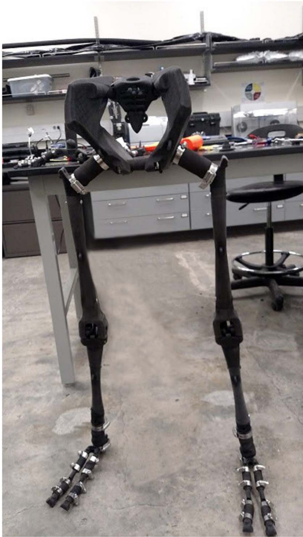
Fig. 1 The fully assembled bipedal robot seen anteriorly without inflation of the synovial joints
