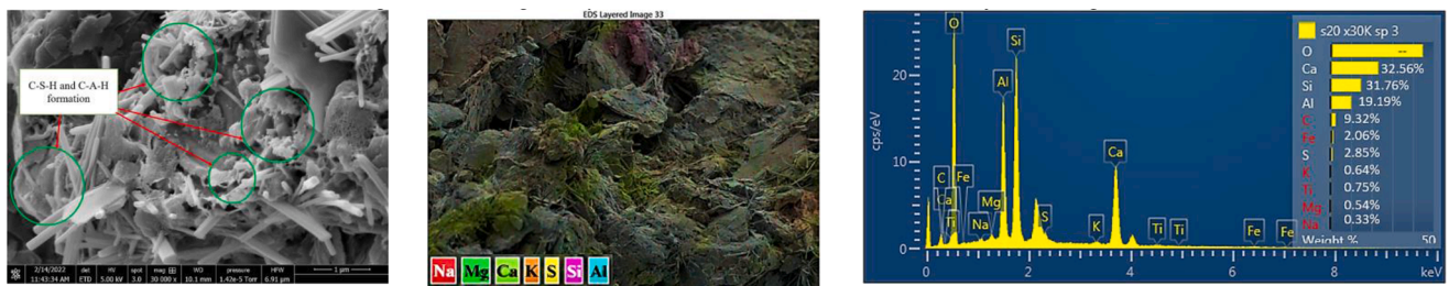
Fig. 6. SEM image, Map and EDX results for ASS2 after 28 days of curing.
