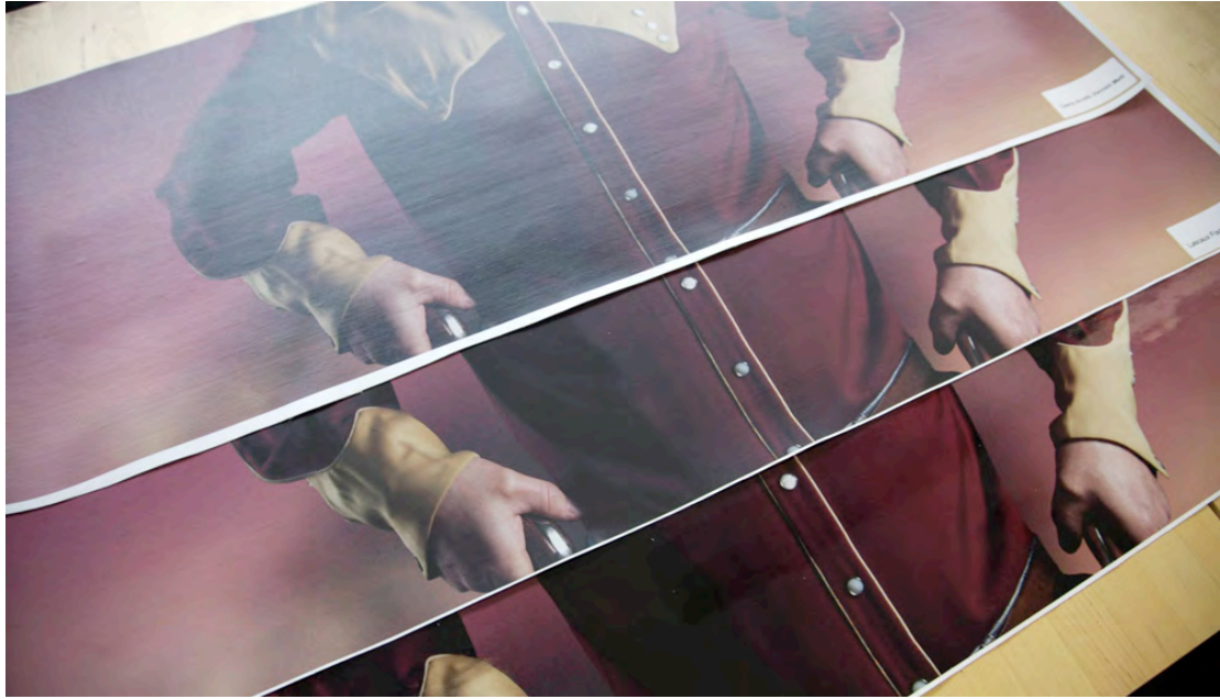
Test strip coating samples for Shock and Awe , (top to bottom coating solutions: Talens Acrylic Varnish Matt, Lascaux Fixativ and Sikkens Autoclear LV Superior) Photograph: Paul Laidler
