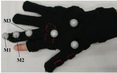
**Figure 5.** Location of the markers on the experiment glove
