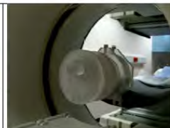
Water phantom set up in SPECT/CT
