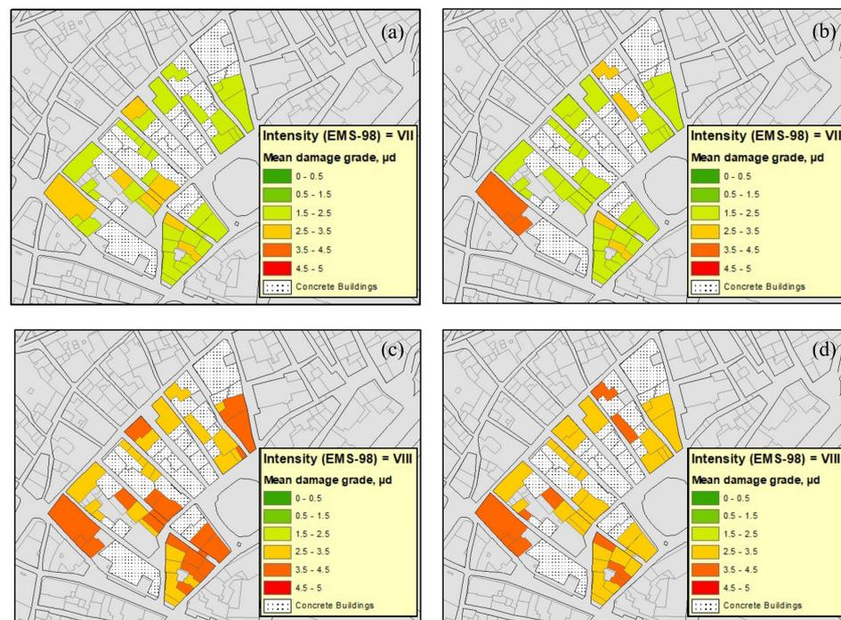
**Figure 19.** Damage scenario for different macroseismic intensities  $I_{EMS-98}$ , considering central values (a,c) and reference values (b,d) of Vulnerability Index  $I_v$ , based on the façade approach.
