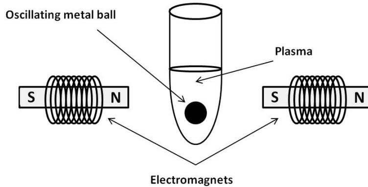
Figure 5. Electromagnetic measurement of clot formation in plasma using 2 electromagnets and a metal ball (Source: Olsen JD; Pennell BJ. Automated Coagulation Systems. In: Haven MC, Tetrault GA, Schenken JR, editors. Laboratory Instrumentation. New York, USA: John Wiley & Sons Ltd.; 1995; 391-409).
