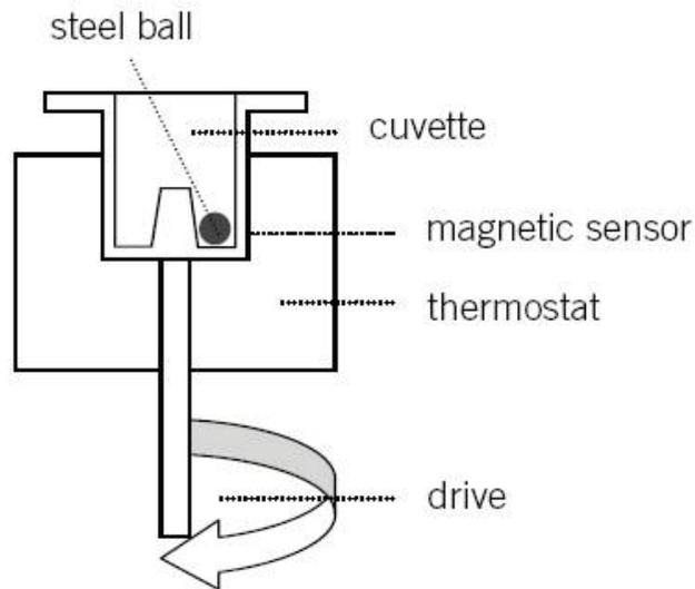
Figure 2. Patented ball technology: mechanical detection of clot formation as used in the KC1 $\Delta$ <sup>TM</sup>/KC4 $\Delta$ <sup>TM</sup> coagulometer. The movement of the metal ball is impeded by the formation of the clot which is returned as the clotting time (Source: Tcoag KC4 Delta Semi Automated Coagulation Analyser, User Manual).
