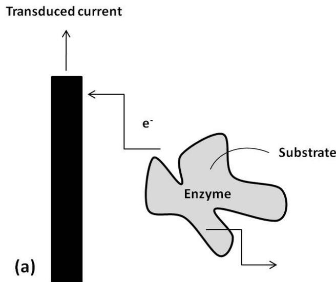
Figure 6. (a) Direct electron transfer between an electrode and an enzyme molecule as occurs in an unmediated amperometric enzyme electrode sensor (Source: Arya SK; Singh SP, Malhotra BD. Electrochemical Techniques in Biosensors. In: Marks R, Cullen DC, Karube I, Lowe CR, Weetall HH, editors. Handbook of Biosensors and Biochips. Sussex, UK.: John Wiley & Sons Ltd.; 2007; 341-393).
