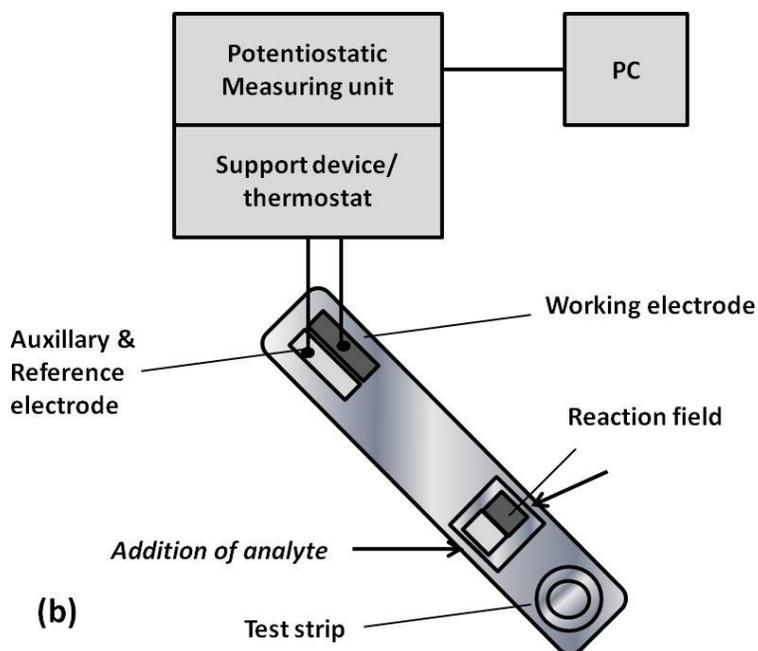
Figure 6. (b) Scheme of a disposable test strip and system for monitoring thrombin generation using chronoamperometric technology (Source: Thuerlemann C; Haeberli A; Alberio L. Monitoring thrombin generation by electrochemistry: Development of an amperometric biosensor screening test for plasma and whole blood. *Clinical Chemistry*, 2009, 55, 505-512).
