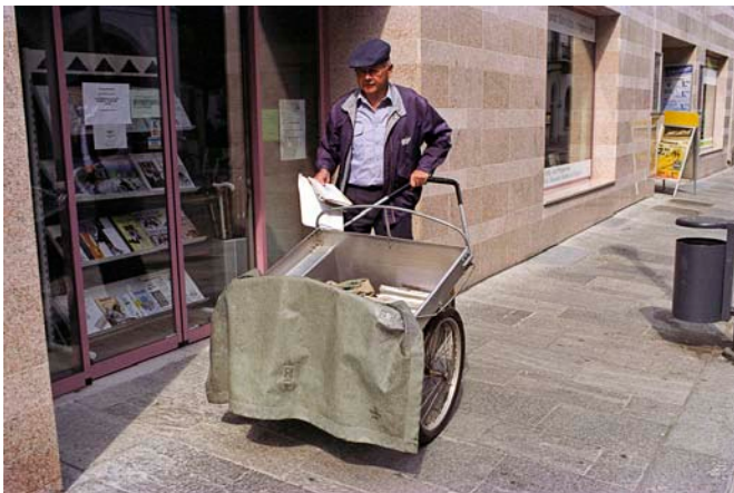
Fig. 7. Battery-powered package cart, Brig, Switzerland
