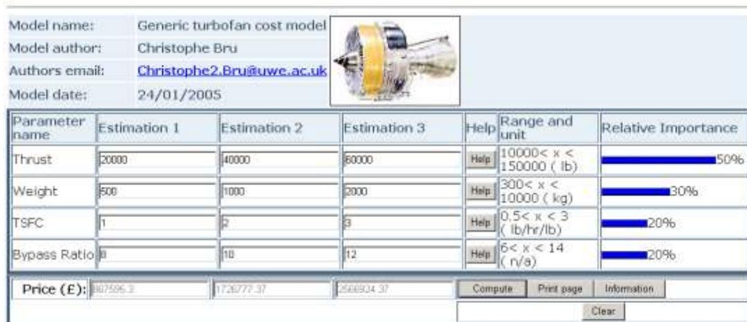
The cost equation is: Price (£) =  $(15.23 * (\text{Thrust} + 32 * \text{Bypass Ratio}) - 13.24 * \text{Weight} - 1.6 * \text{Power}(\text{TSFC}, 2)) * 2.874$
