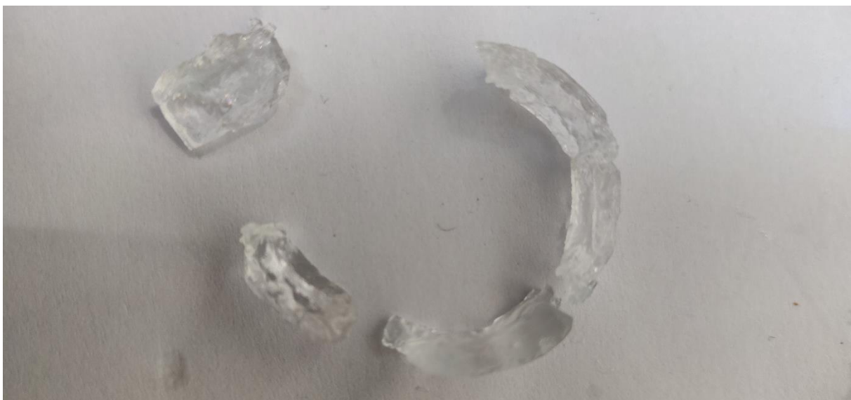
Figure 4: Sugar crystals grown in ring mould over 8 days.
