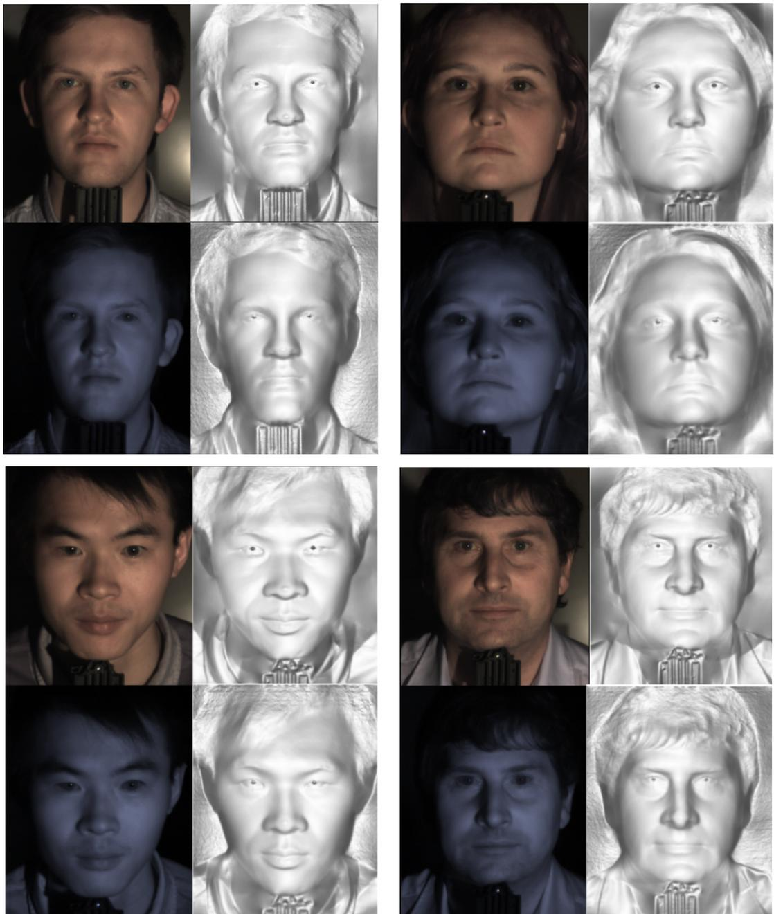
Figure 3.4: Example raw images and reconstructions using visible (top) and NIR light sources for four subjects. For these experiments only, the subjects were asked to rest their chin on a support in order to ensure that all subjects are compared to each other in fair conditions. Note that hair is well recovered (other methods e.g. 3dMD tend to reconstruct hair poorly).
