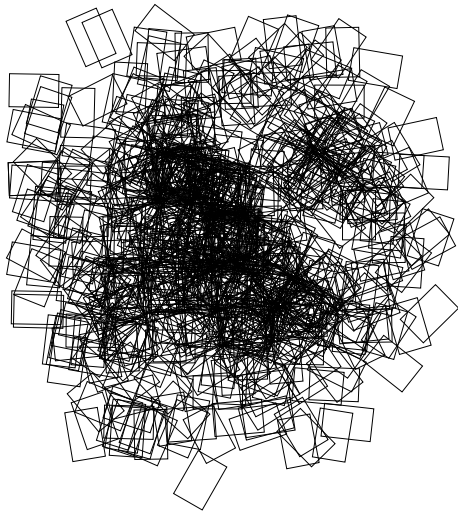
Figure 12: Montage showing the collection of inferred tables from each independent robot pose, for very noisy ( \sigma_r = 0.5, \sigma_\theta = \pi/8 ) sensors.
