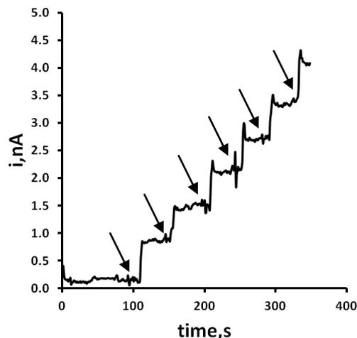
Figure 7. Chronoamperometric investigations of GSH at a microband CoPC-SPCE electrode in MEM dilute 1:1 with 0.2 M phosphate buffer solution, pH 7.4 at 37 °C. Arrows represent additions of 5  $\mu\text{L}$  102 mM GSH into 8 mL quiescent (stirred only to mix for 10 s).
