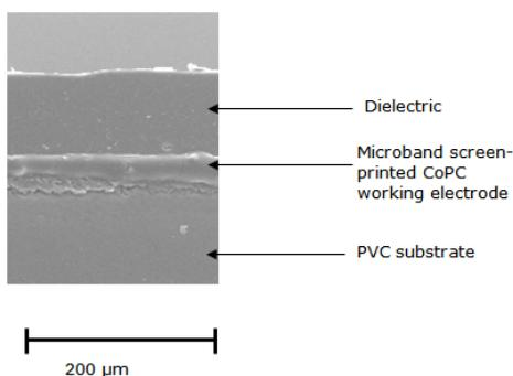
Figure 2. Scanning electron micrograph of a microband CoPC-SPCE.
