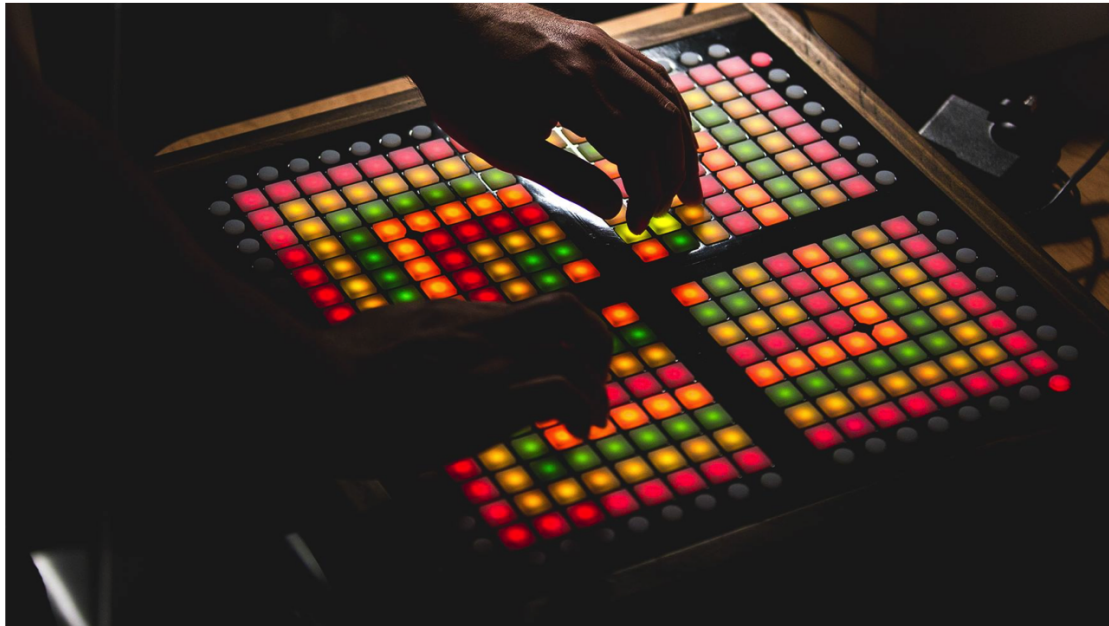
Fig. 1. Large format grid controller, made from 4 smaller grid controllers
