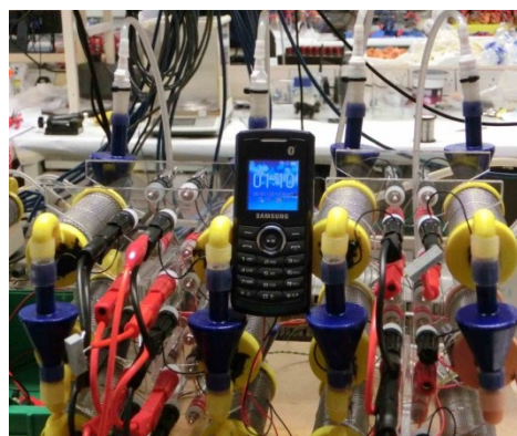
Fig. 5 Samsung GT-E2121B powered by the ceramic MFC stack
