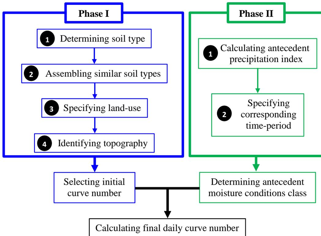
Figure 5. Steps to be followed for calculating daily curve number. Here, Phase I consists of determining the initial curve number ( $CN_i$ ), whereas Phase II consists of determining the antecedent moisture conditions class.
