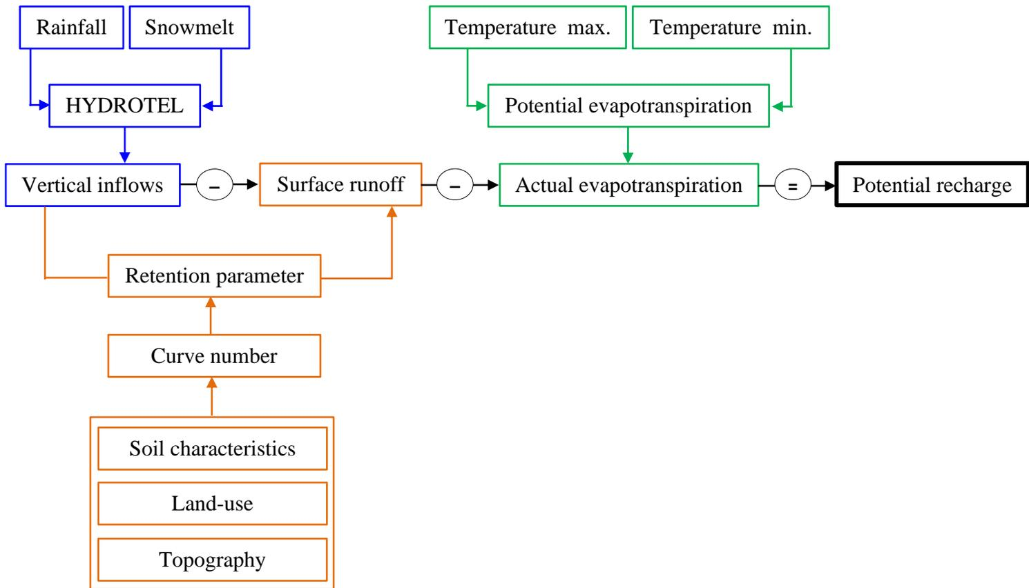
Figure 3. Procedure for computing the annual PGR using water budget method.
