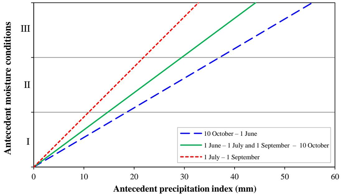
Figure 7. Chart for determining AMC class according to API and time-period (Adapted from Monfet (1979)).
