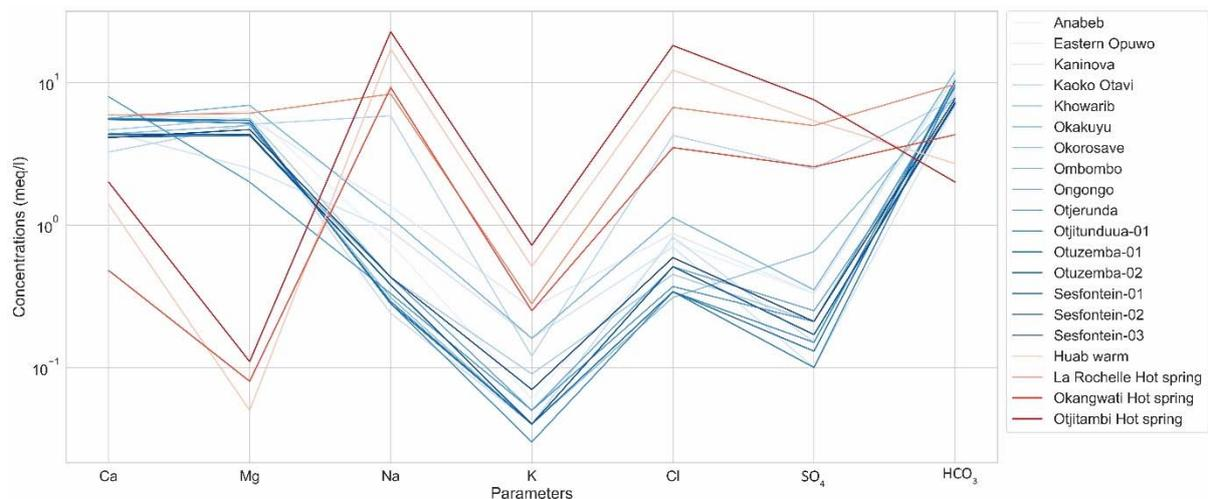
**Figure 6.** Schoeller diagram of groundwater from springs (blue) and thermal springs (orange and red) sampled in this study.
