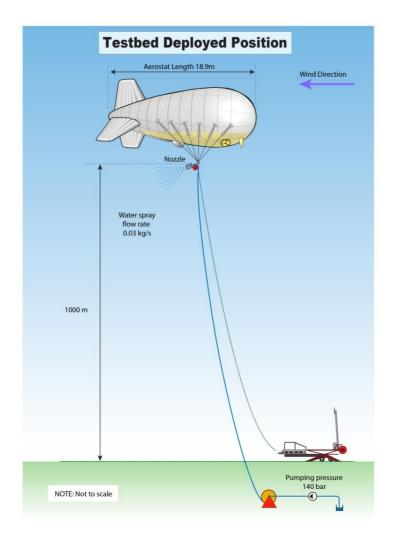
Figure 1. The proposed testbed for investigating tethered-balloon technology. (Copyright reserved, Kirsty Kuo, University of Cambridge).
