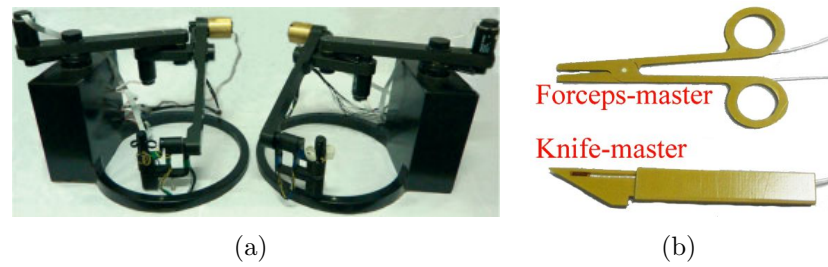
Figure 2.23: ‘Microhand A’ (a) mechanical master and (b) forceps-master and knife-master (Sang et al. (2011); Zhang et al. (2013), ©2011,2013 by John Wiley & Sons)
