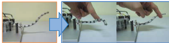
Figure 2.29: 4-DOF flexible continuum robot (reprinted from Yoon et al. (2010) with permission from the authors)
