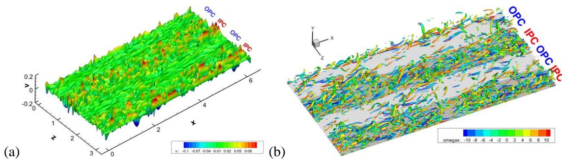
Figure 1: Instantaneous normal velocity at wall (a) and turbulent coherent structures (b) in the channel with SADS.
