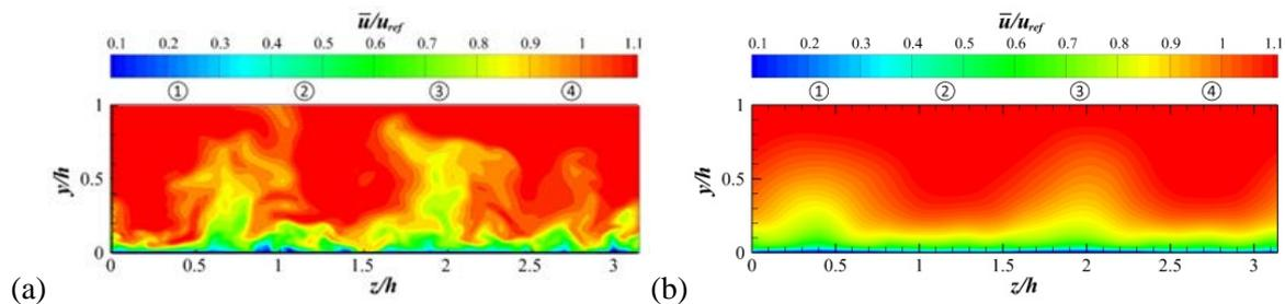
Figure 2: Instantaneous (a) and mean streamwise velocity (b) in the channel flow with SADS. The characters of ① & ③ and ② & ④ represent the regions of OPC and IPC, respectively.
