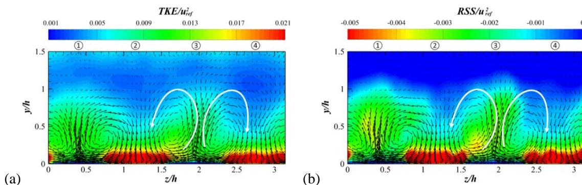
Figure 3: Turbulent kinetic energy (a) and Reynolds shear stress (b) as well as mean velocity vectors in the channel flow with SADS. The white arrows represent the local sweep and ejection motions.
