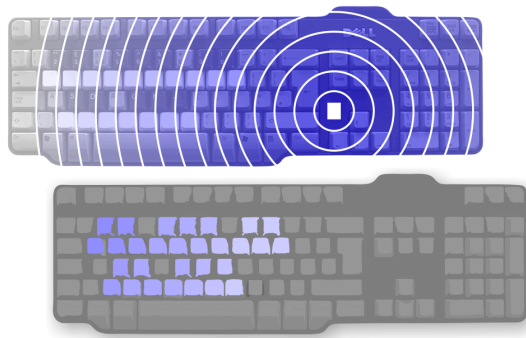
Figure 8. Pressure Sensitivity (top) and Compensation Map (bottom).
