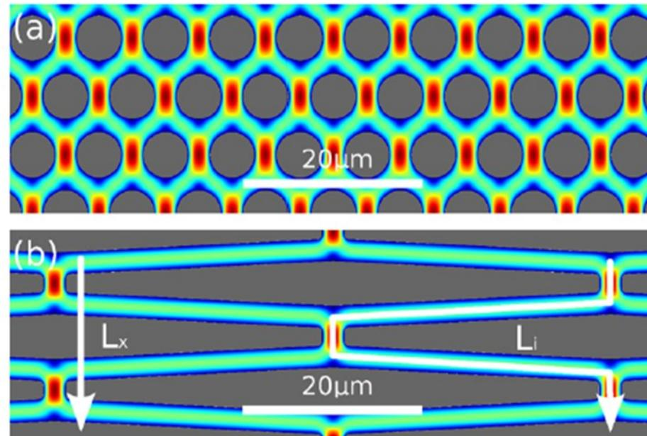
Top view of pillar arrangement and velocity field of (a) a conventional cylindrical pillar array column and (b) a radially elongated pillar column. The white arrow  $L_x$  indicates the net direction of flow; white arrow  $L_i$  indicates the direction of flow along the tortuous path followed by the liquid.
