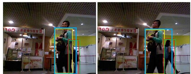
**Fig. 7** Occlusion search region:  $\Gamma_{search}^i$  (blue line),  $\Gamma_{occ}^i$  (yellow line),  $\Gamma_{obj}^i$  (red line),  $\Gamma_{KF}$  (green line)
