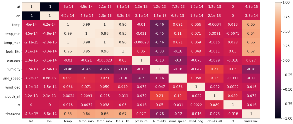
Figure 6: Distance matrix of weather parameters using Pearson's correlation. A strong correlation can be noticed between “temp”, “temp_min”, “temp_max”, “wind_speed”, “wind_degree” and “feels_like”. There is also a discernible correlation between “clouds_all” and “humidity”/“windspeed”.
