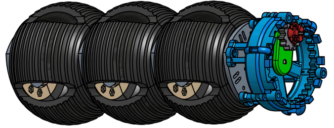
Fig. 14. Side view of robot worm design showing the front gear mechanism and soft body worm segments.
