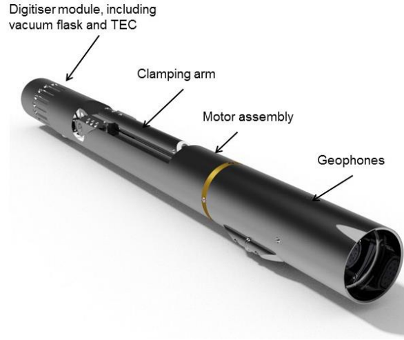
Figure 1 A picture of the GSR tool housing the electronic module and TEC.
