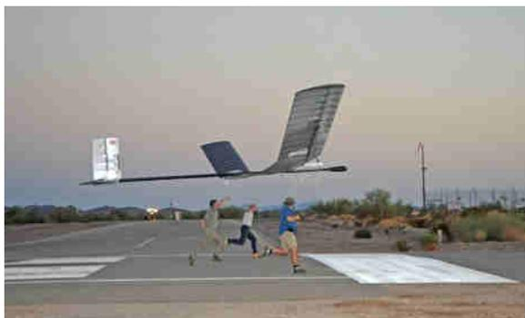
Figure I.3: *Qinetiq Zephyr*, a solar-powered, 18 metres-wingspan-UAV, which sustained flight for two weeks in July 2010.
