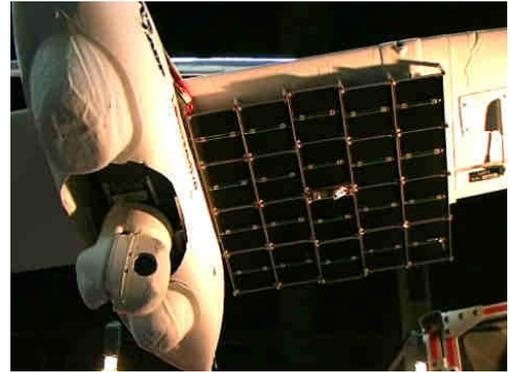
Figure I.2: Photovoltaic panels installed as a laser receiver unit under the right wing of the 3 metres-wingspan *Lockheed Stalker*.
