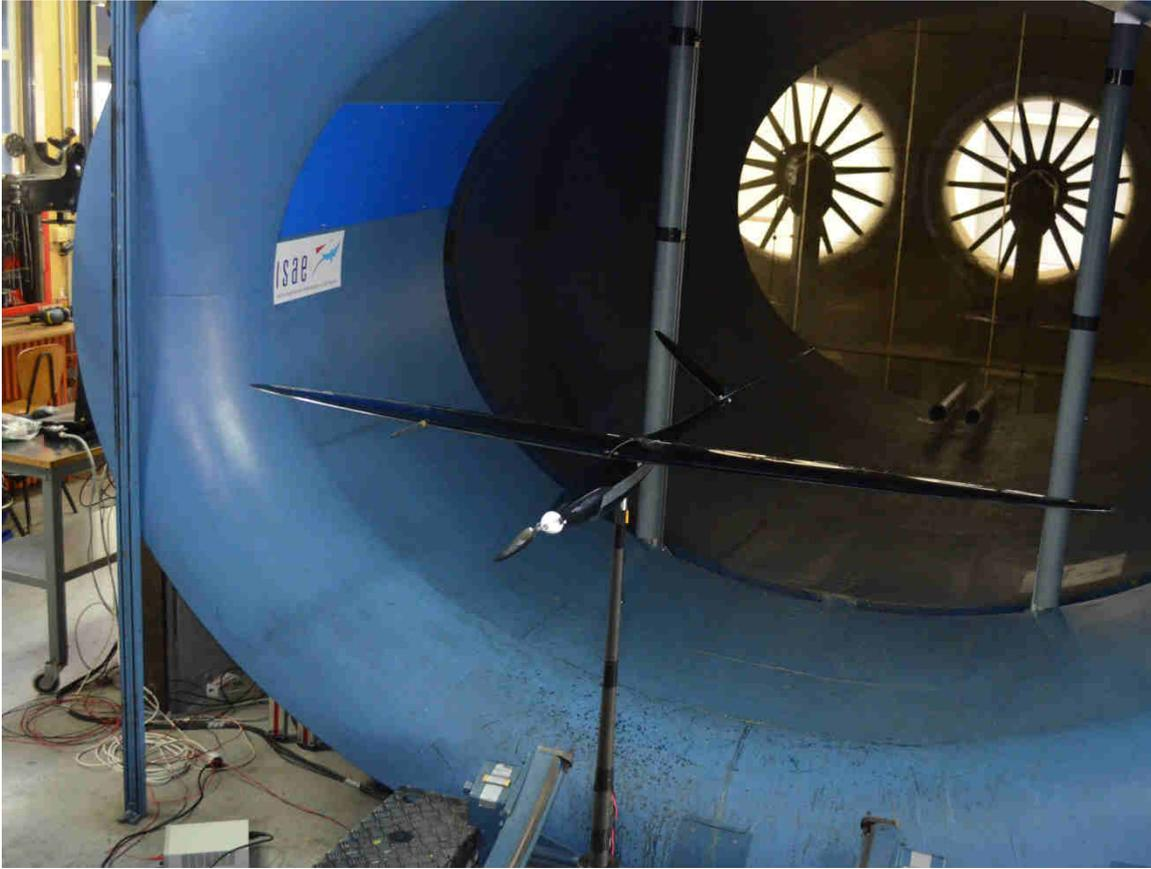
Figure III.5: The *DT-18* experimental mock-up into place, through the single ventral mast, inside the elliptical test section of the *S4* wind tunnel. The open test section is clearly visible, as the workshop is visible (left) outside of the section. The suction fans are visible (top right) at the end of the suction chamber, leeward of the diffuser. The curved rails of the cradle can also be seen (bottom), as well as the external feed (bottom left) for powering on board electronics.
