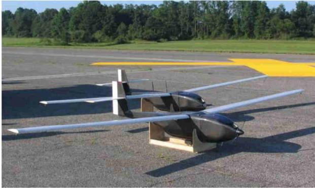
Figure I.1: *Ion Tiger*, a fuel-cell-powered, 5.15 metres-wingspan, which sustained flight for 48 hours in April 2013 [9] using liquid hydrogen.
