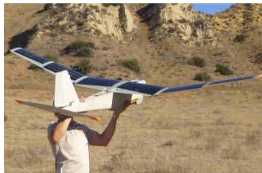
Figure I.4: *Aerovironment Puma AE*, a solar-powered, 2.8-metres-wingspan, which sustained flight for up to 9 hours in August 2013.
