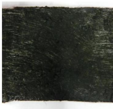
*Figure 2.3. MPL (Microporous layer) on carbon veil used as single layer electrode.*
