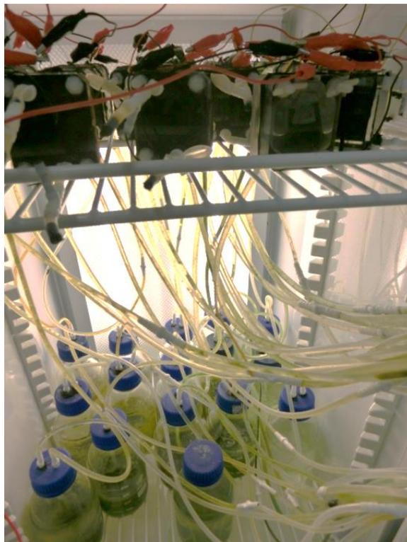
*Figure 4.5 MFCs and bioreactors in temperature controlled light incubator.*
