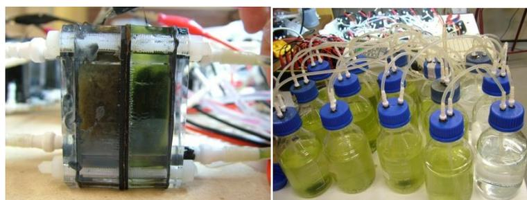
*Figure 4.1 Experimental set-up; two-chamber microbial fuel cell with biotic cathode (left). Photoreactors and control bottles connected to the cathodic side of tested MFC (right).*
