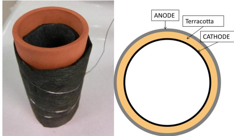
*Figure 2.6 Novel design of inverted tubular MFC with anode wrapped around the outside of the terracotta tube.*
