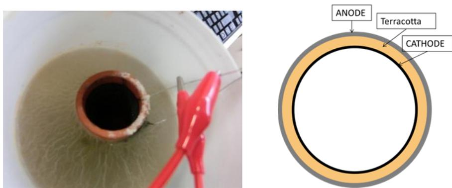
Figure 5.26 Immersed MFC with anode outside and cathode inside the ceramic tube (left) and MFC diagram (right).
