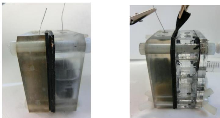
*Figure 5.1 Experimental set up. Left: control MFC with carbon veil electrode in the cathode half-cell, right: single layer MPL coated carbon cloth pressed against the membrane.*
