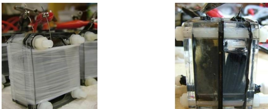
*Figure 2.5 Single-chamber MFC with open to air cathode (left) and two-chamber MFC with aqueous cathode (right).*
