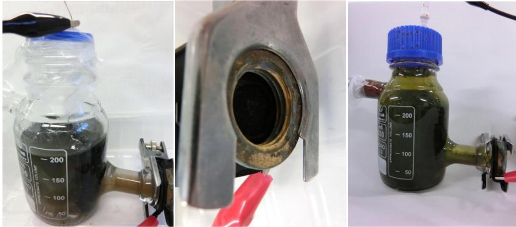
*Figure 9.1 H-type fuel cell (left), MPL as cathode/membrane assembly (centre), H-type fuel cell after 2 months of operation (right).*
