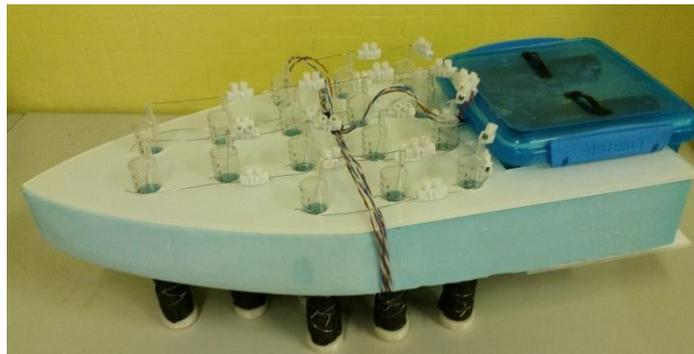
*Figure 6.1 MFCs as part of the floater design for practical implementation into the wastewater treatment tank.*
