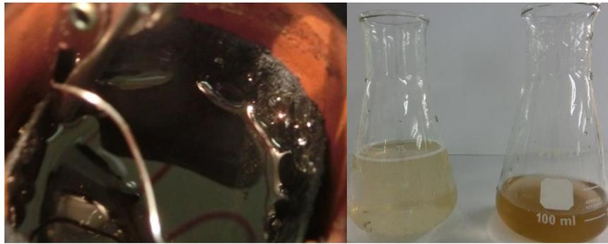
Figure 5.37 Catholyte formation (left) and the amount of water produced in working (under  $53 \Omega$  resistor) and OCP conditions (right).
