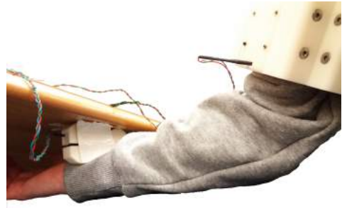
Fig. 7: Upper arm experiments, supported forearm closes switch during elbow flexion.
