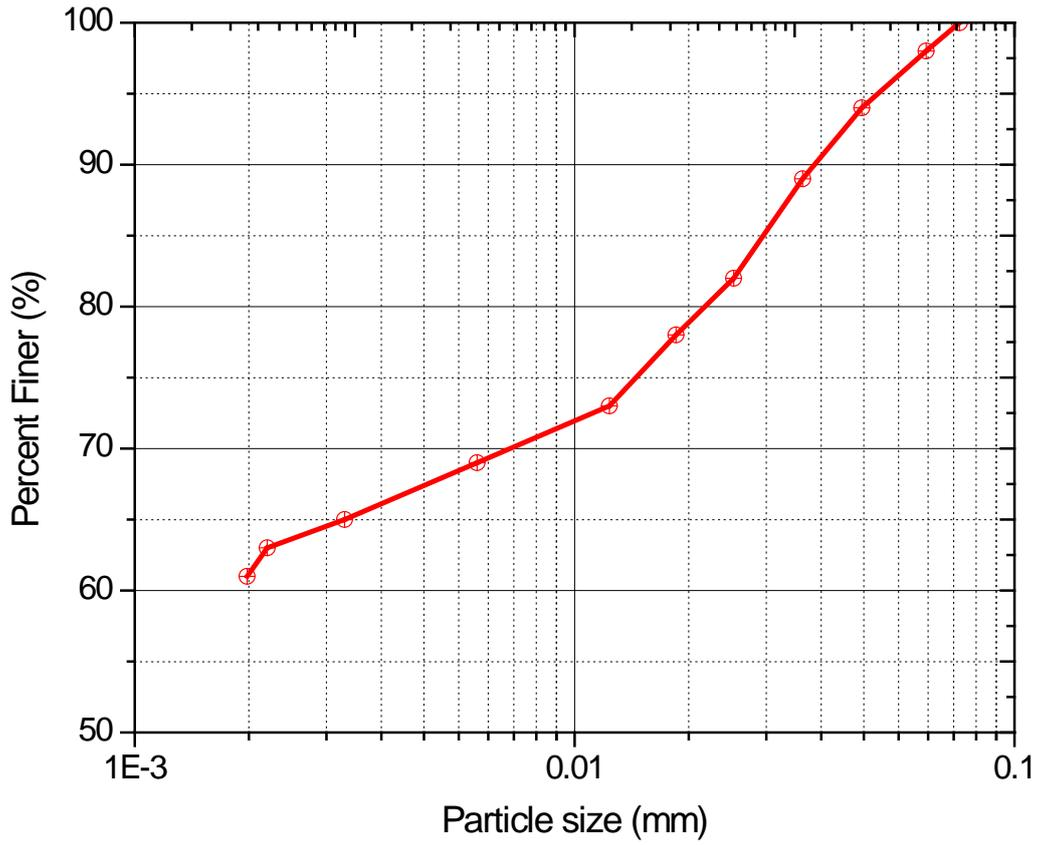
Figure 1. Particle size distribution of the clay
