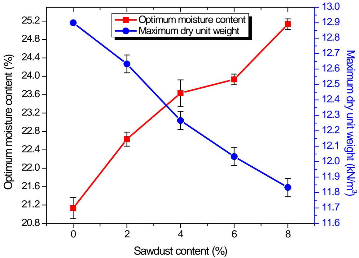
Figure 7. Variation of compaction characteristics of the bentonite with sawdust
