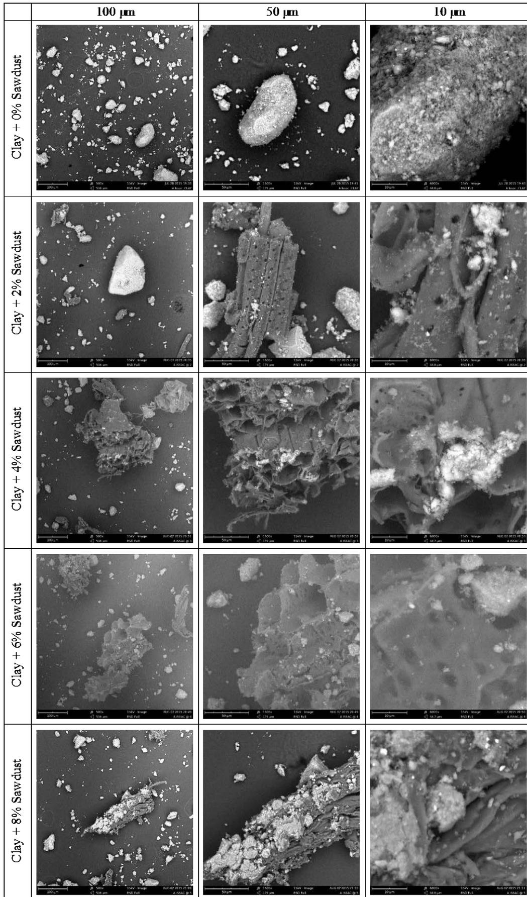
Figure 10. SEM micrograph of the clay with sawdust
