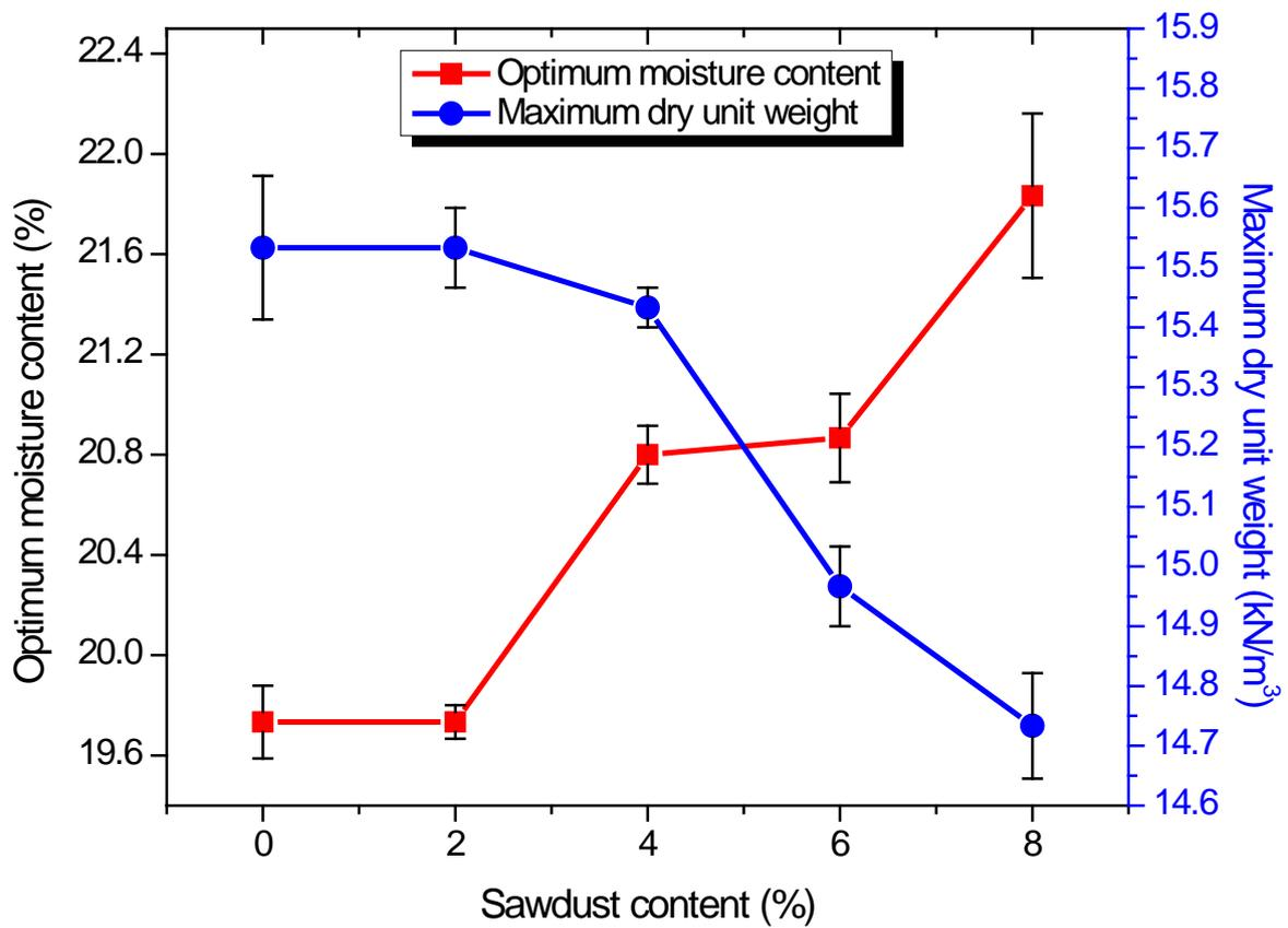
Figure 6. Variation of compaction characteristics of the clay with sawdust
