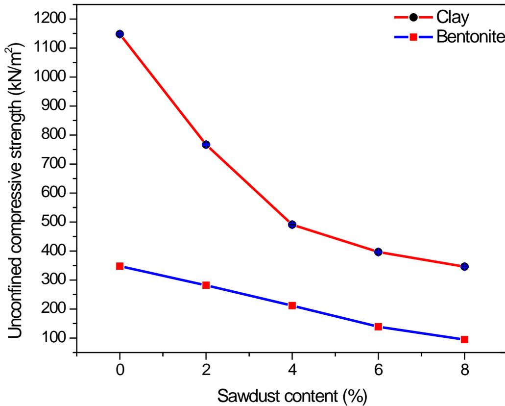
Figure 8. Variation of UCS of the clay and bentonite with sawdust
