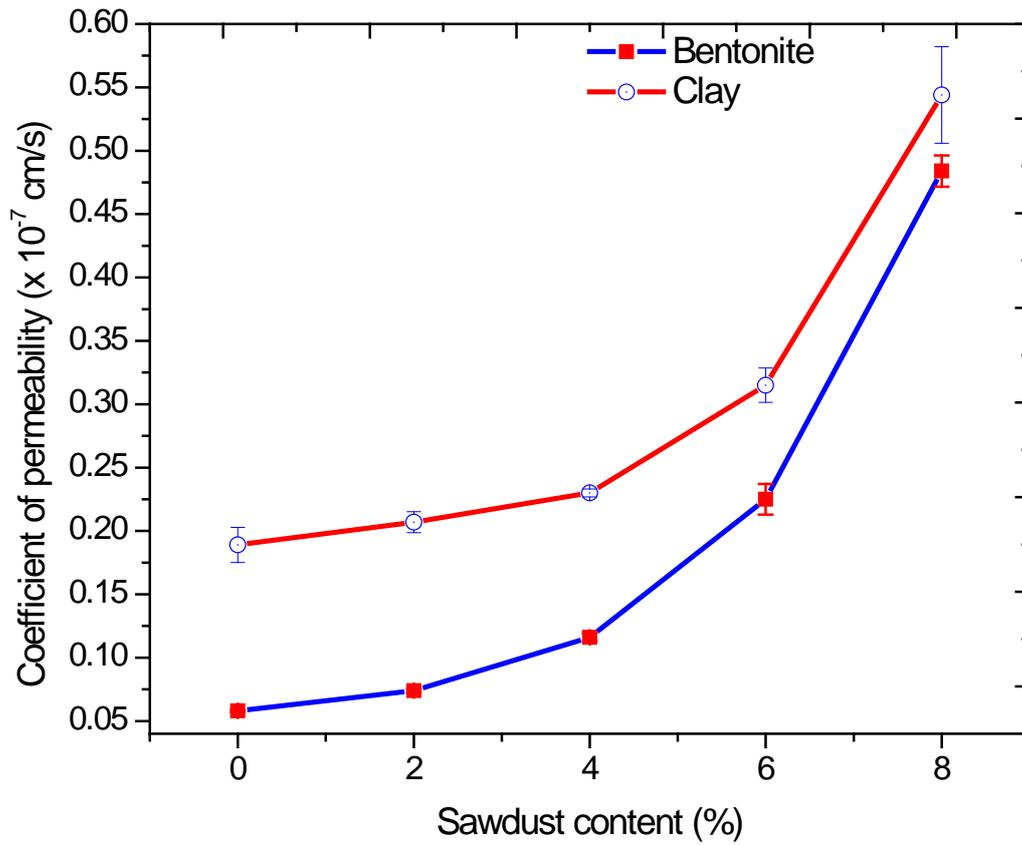
Figure 9. Variation of permeability of the clay and bentonite with sawdust
