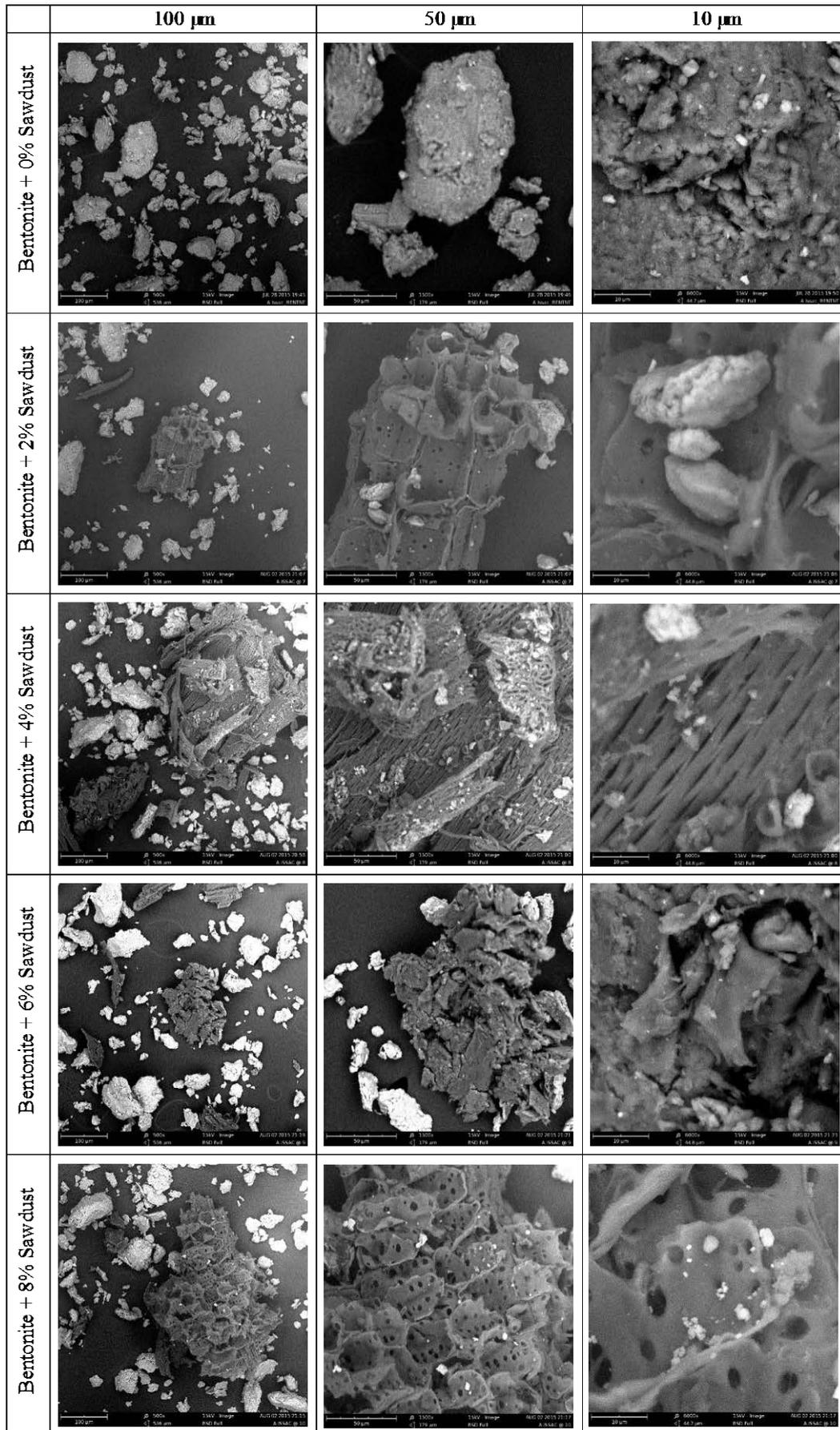
Figure 11. SEM micrograph of the bentonite with sawdust
