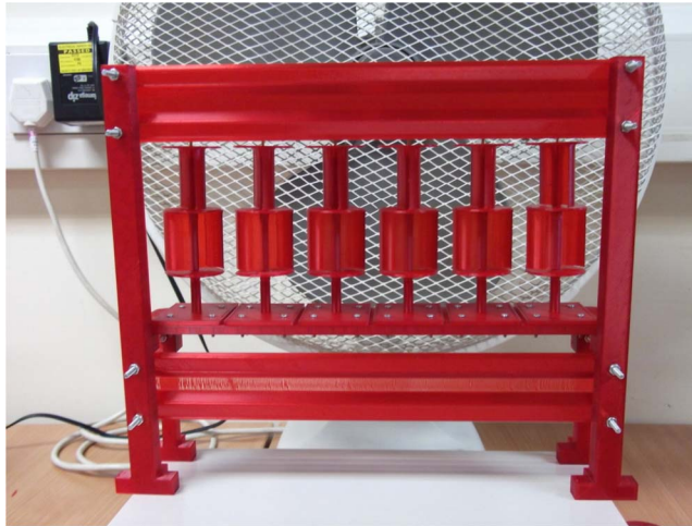
Figure 6. Experimental setup with six VAWTs. Frame width 275 mm, height 235 mm. Vertical support pillars 10 \times 15 \times 235 mm. Upper and lower crossbars each with height 40 mm, thickness 1 mm, and protruding 8 mm. VAWTs freely rotate on rigid metal pins 1 mm in diameter and positioned 42.5 mm adjacently.
