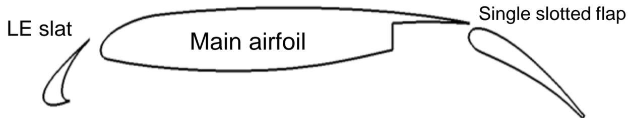
**Fig. 1** The 30P30N three-element airfoil (Klausmeyer, 1994)
