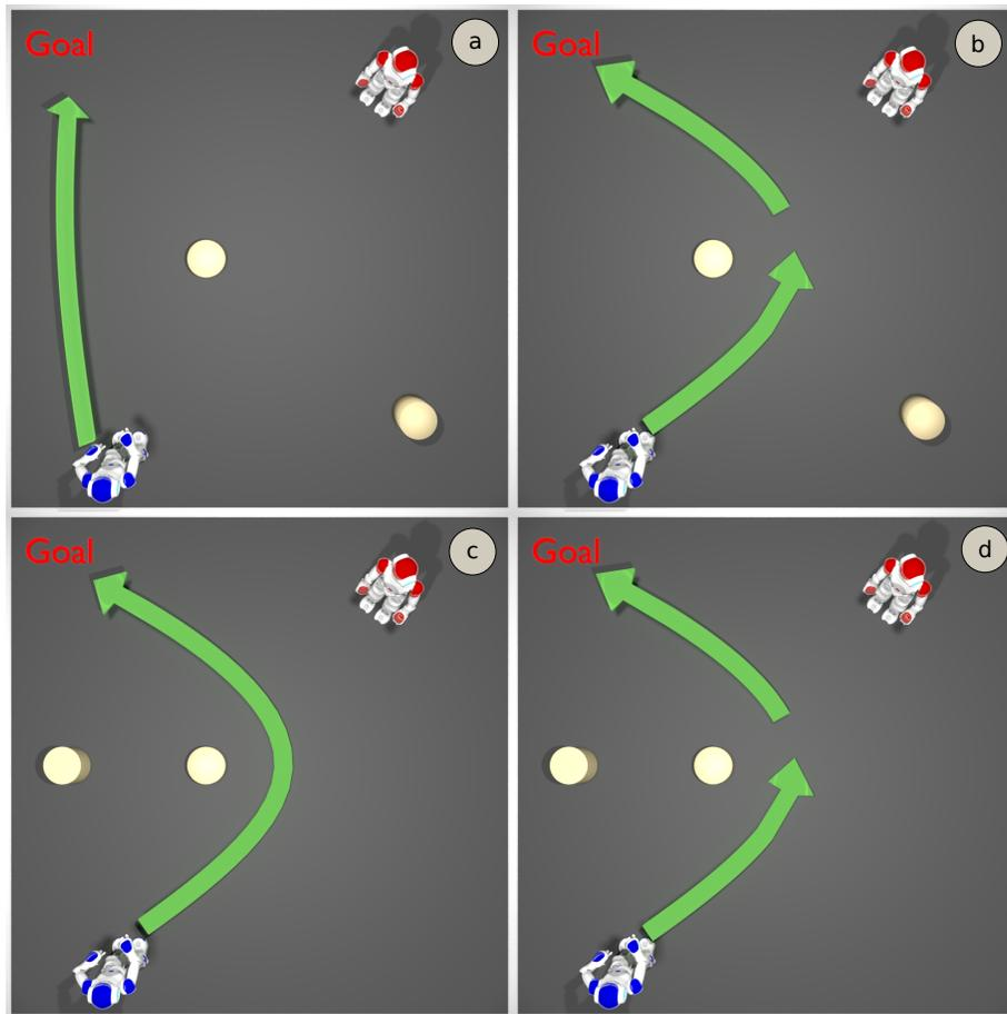
Figure 3: Illustration of the four conditions in experiment 1. The blue robot is the demonstrator. The red robot is the imitator. The green arrows depict the path taken by the demonstrator. Note that in panel c the demonstrator cannot pass between the two round obstacles. Details in text.
