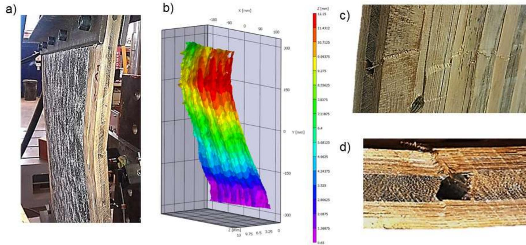
Figure 8. G-XLam3 panel discarded for buckling failure during compression test using DIC. a) Failure of panel mounted on the test machine b) 3D-Strain map of the failure c) Detail of the failure area. d) Detail of the shear failure produced by the buckling effect during compression test.
