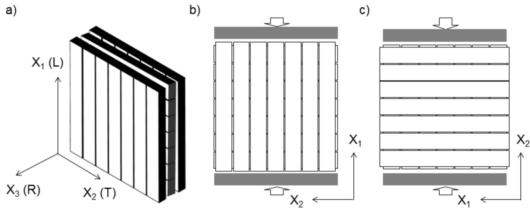
Figure 1 a) Geometric ( $X_1$ ,  $X_2$ ,  $X_3$ ) and orthotropic (L, T, R) axis of the G-XLam panels b) Diagram of the compression test in the longitudinal direction of the panel c) Diagram of the compression test in the transverse direction of the panel.
