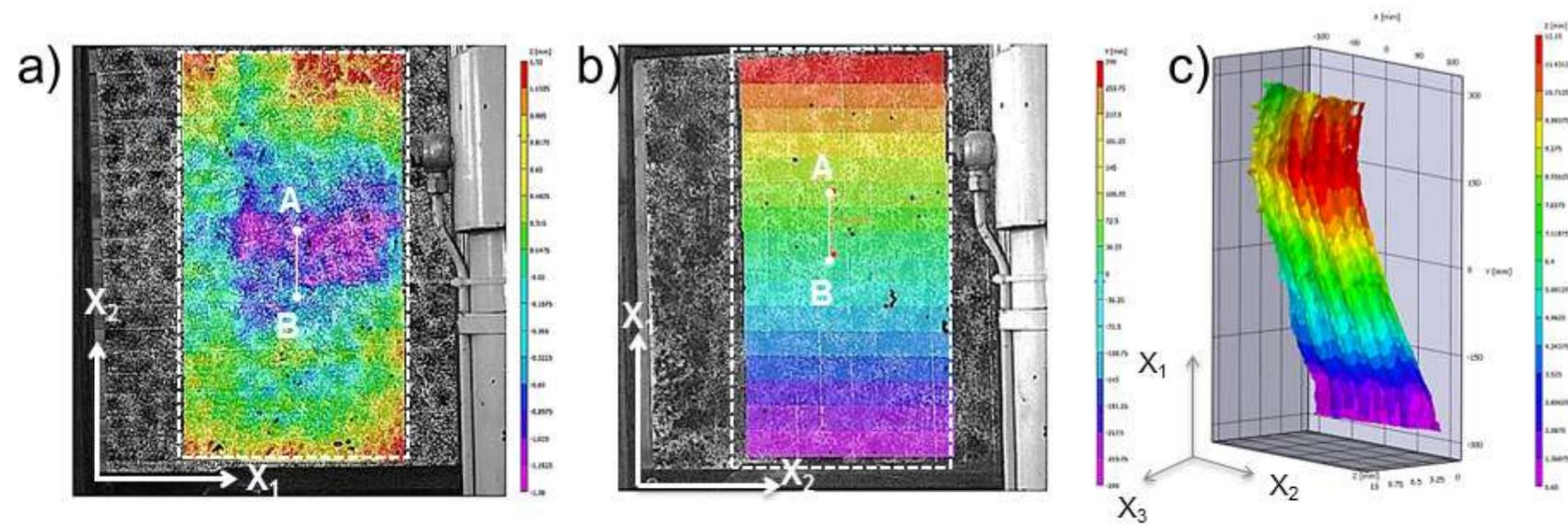
Figure 4. Setup for the compression test of CLG panels using the DIC method.
