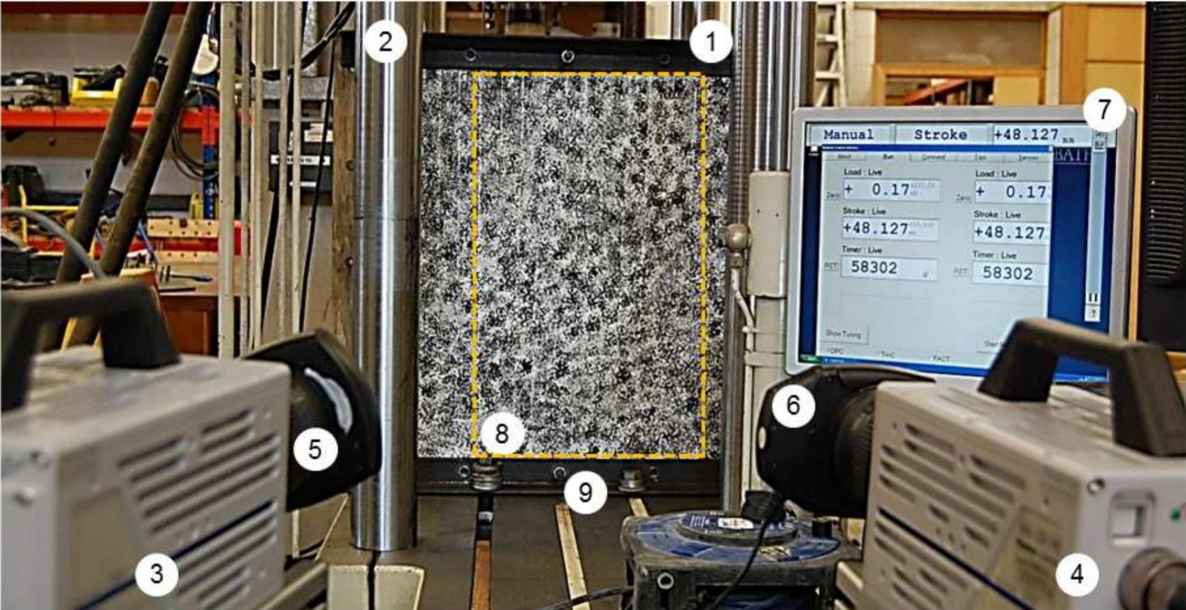
1. Object: G-XLam panel. 2. Mayes 20kN test machine. 3. Master camera. 4. Slave camera.
