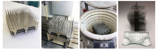
Figure 1: Preliminary exploration of the RPT system for glass thermoforming, photos: T. Jørgensen, 2010.
