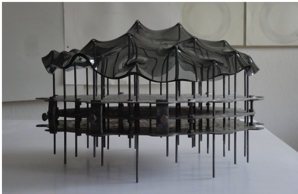
Figure 3: RPT system with glass bowl (upside down) still resting on the pins following the slumping process, photo: T. Jørgensen, 2012.
