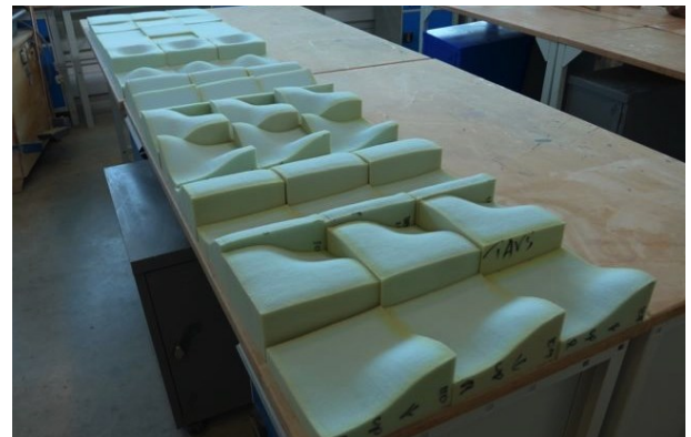
Figure 10: Foam shapes produced for empirical testing of the tooling system's performance, photo: T. Jørgensen, 2014.
