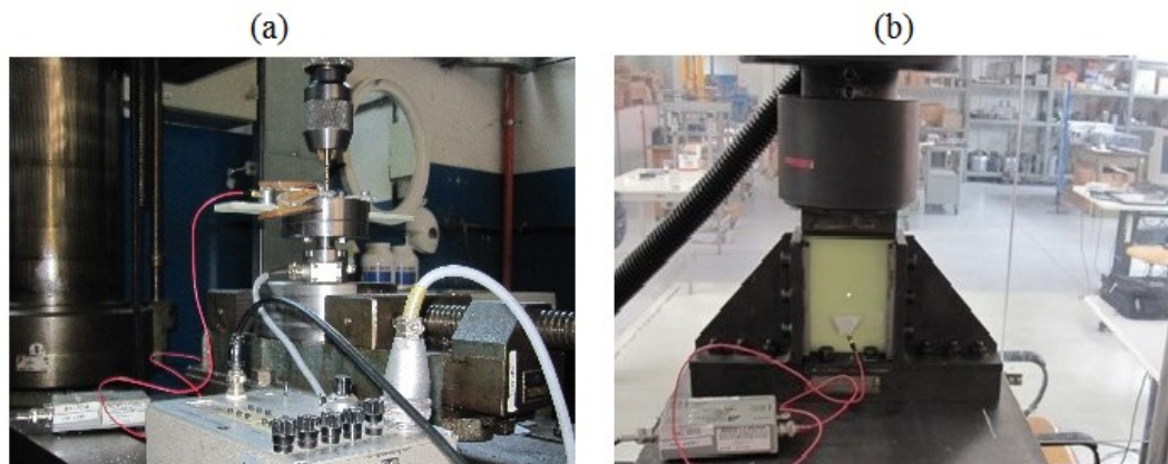
Figure 2. Experimental setup (a) drilling, (b) compression.
