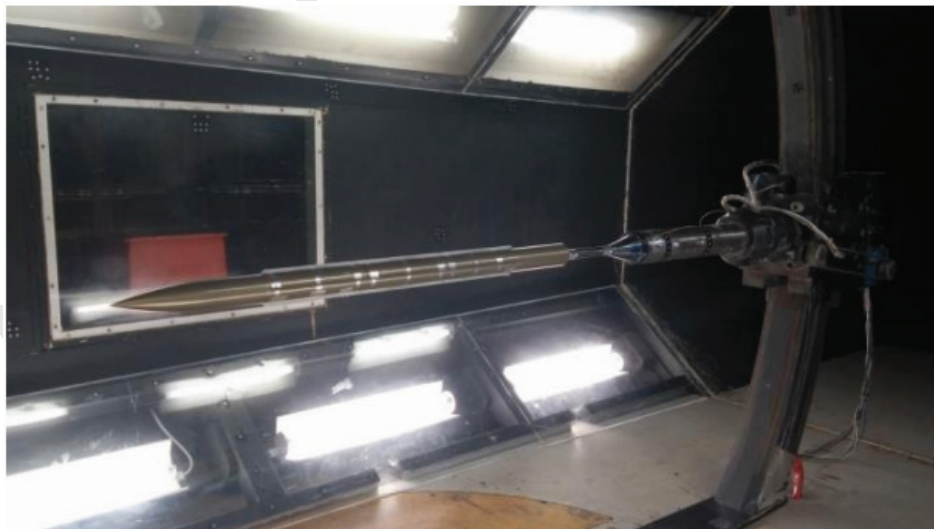
Fig.3: Model Setup in the low speed wind tunnel
