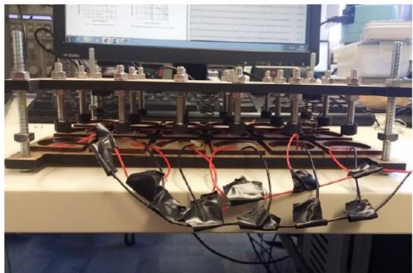
Figure-9. Prototype Harvester side-on view with piezo sensors
