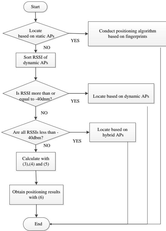
Fig. 3. Algorithm Process The workflow of HAPLA
