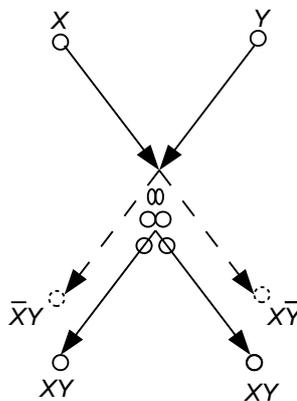
Figure 1: Margolus gate: collision between soft balls.
